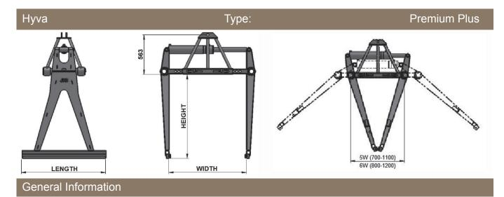
Hyva Premium Plus, light weight brick clamp is suitable for all palletized and non-palletized construction materials.
