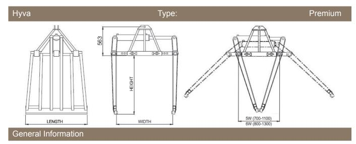
Hyva Premium brick clamp is suitable for all palletized and non-palletized construction materials.
